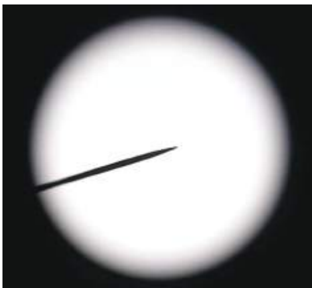
Figure 3. Microscope eyepiece with pointer. This technique is more common in the traditional microscopy classroom to point structure of interest [Online image] (2018). Retrieved from https://www.amscope.com/wf10x-microscope-eyepiece-with-pointer-23mm.html .
