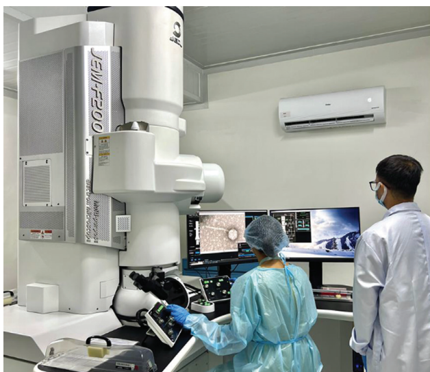
Figure 1. JEOL JEM-F200 Transmission Electron Microscope installed at the Research Institute for Tropical Medicine.
